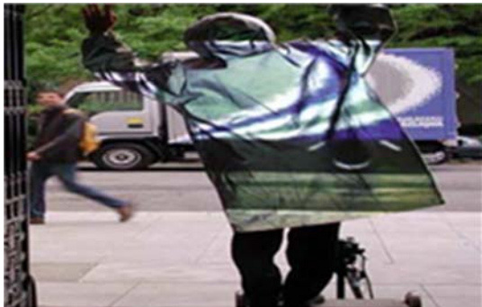
Figure 10. RPT with projection on a retroreflective cloak (2003).
